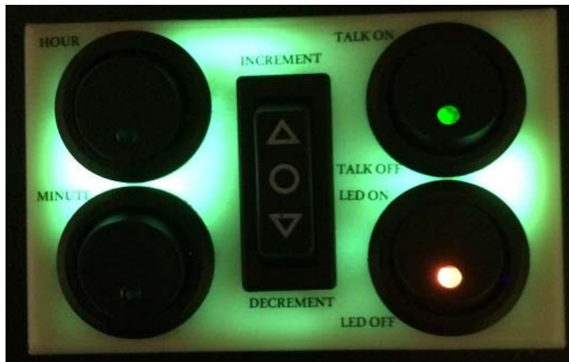
Figure 5.153 – Pushbutton Panel with LEDs On
