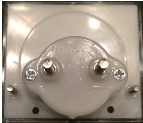
Figure 5.101 – Rear of meter with LED mounting holes
