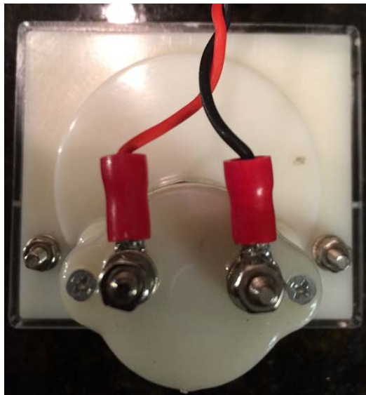
Figure 5.113 – Ring Terminals Installed
